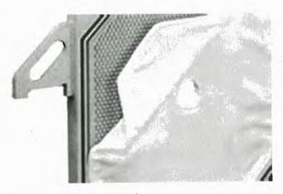
When multiple filtering plates are pressed together, they form a filter housing. Filter media (diatomaceous earth (DE)), is applied to the cloths. As waste water flows through the filter media, suspended solids are collected on the filter media.
