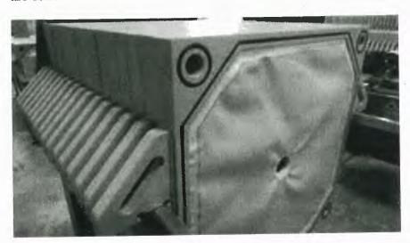
Once a sufficient amount of suspended solids are collected on the filter media, a significant pressure drop occurs through the filter press. At this time the collected solids along with the filter media must be removed. To remove the solids and filter media, the filter press is opened and the individual plates are separated. If needed, the filter plates are removed from the filter press and transported to another location.
